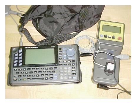
The CBL (shown above) is a portable data acquisition unit that connects to calculators for easy readout of data. A "single-axis, low-g" accelerometer attaches to the CBL to measure forces that give rise to accelerations between 0 and 5 times the acceleration due to gravity (5 g's). The CBL and accelerometer fit in a waist pack for safe transport on the midway rides.
