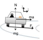
**Solution** Given r = 30.5 m,  $\mu_k = 0.6$ . For the horizontal forces - the centripetal force (effect) is provided by friction (cause), which keeps the car from sliding or having any negative lift. For vertical forces - the normal force and weight of the car are equal and opposite. We can write the equations of motion. Solve for v by re-arranging the equations below, substituting for  $a_c$  and  $F_k$ .
