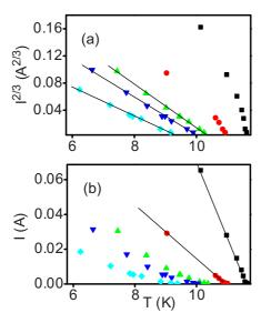
FIG. 2. (Color online) (a) Two-thirds power of the applied current vs the temperature for sample B for the following normalized-resistance criteria:  $R_c/R_n = 0.49$ , 0.62, 0.69, 0.81, and 0.92 (where  $R_n$  is the normal-state resistance). (b) The same applied-current data plotted linearly against the same temperatures as in panel (a). Straight lines are guides to the eye.
