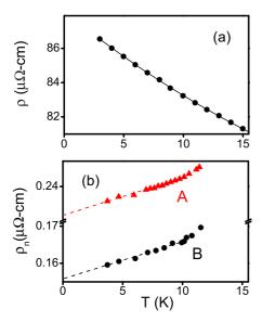
FIG. 4. (Color online) (a) Resistivity of pure FeTe deposited on ZnSe/GaAs without any Bi<sub>2</sub>Te<sub>3</sub> top layer. (b) Intrinsic normal-state resistivity of the interface for samples A (red triangles) and B (black circles).
