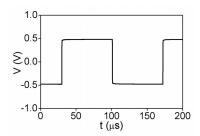
FIG. 2: Waveform of voltage at loudspeaker terminals, recorded at a  $200~{\rm MS/s}$  sampling rate.
