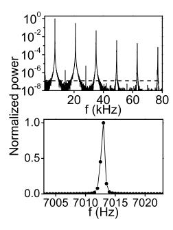
FIG. 3: Power spectrum of the (unaveraged) acoustic output of one loudspeaker at a distance of 0.7 m. The power coefficients are normalized w.r.t. the fundamental peak. (a) Log-linear plot of the 20 Hz-80 kHz window in 20 Hz steps taken at a 2MS/s sampling rate. The horizontal dashed line corresponds to the absolute sound level of 0 dB SPL. (b) Linear-linear plot of the region near the fundamental peak in 0.5 Hz steps taken at a 50 kS/s sampling rate.
