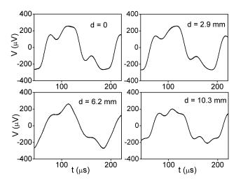
FIG. 4: Acoustic waveforms measured at the listener position for four displacements. The d=0 curve corresponds to the control stimulus (which is essentially twice the waveform produced by just one speaker). The waveforms were recorded at a 20 MS/s sampling rate.
